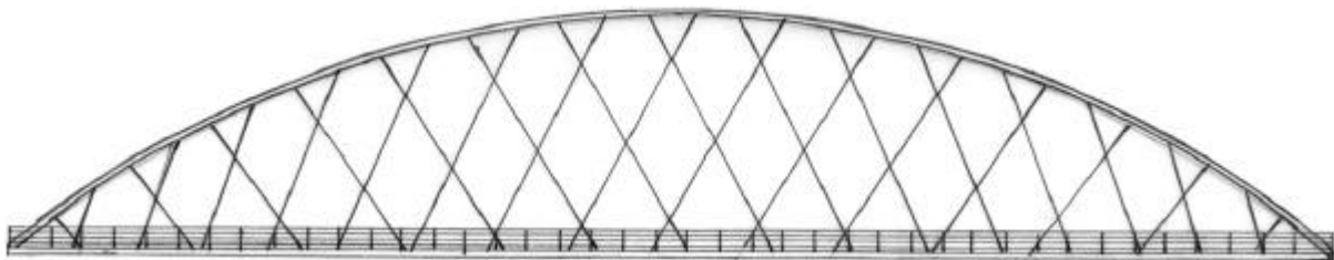
Fig. 5. Bolstadstraumen Bridge built in western Norway in 1964. Rise of arch 0.18 times span.
