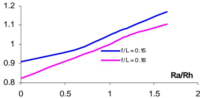
Fig.8 Evolution of arch compression with  $f/L$
