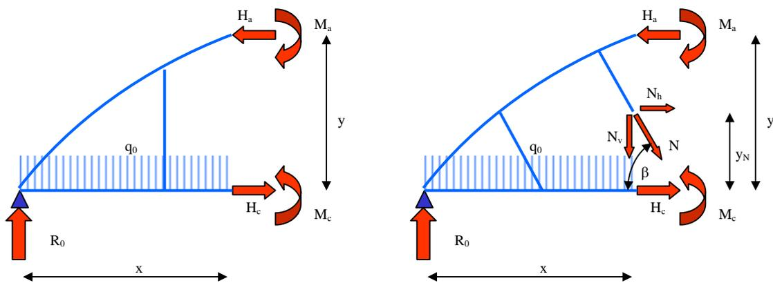
Fig 2. Equilibrium vertical hanger arch (left), fan arranged hangers (right)
