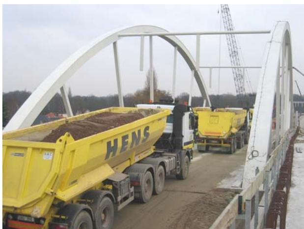
Fig.10 full scale tests of the railway bridges near Antwerp with heavy lorries
