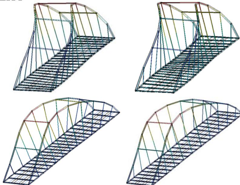
Fig.7 : Arch buckling shapes
