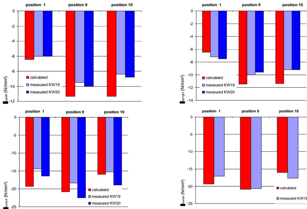
Fig.11 Longitudinal stresses at upper (above) and lower flange of the arches
