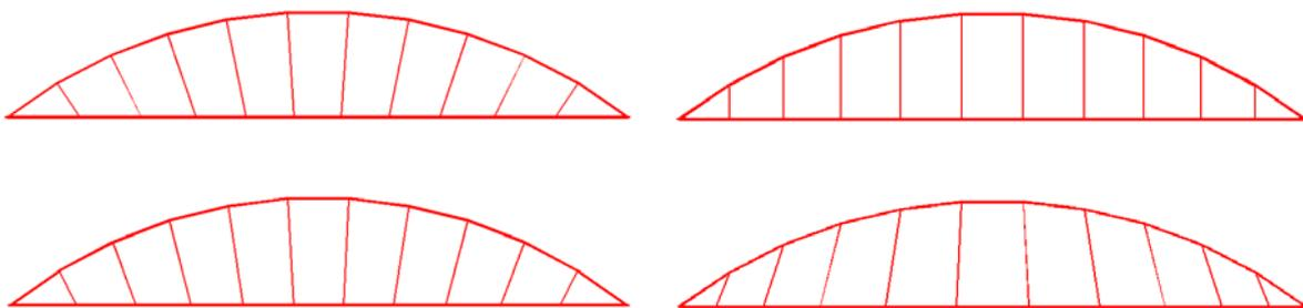
Fig. 1 : Various hanger arrangements and values of  $R_a / R_c$
