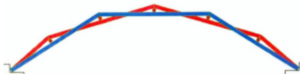
Figure 13: Schematic representation of Rainbow Bridge structure.
